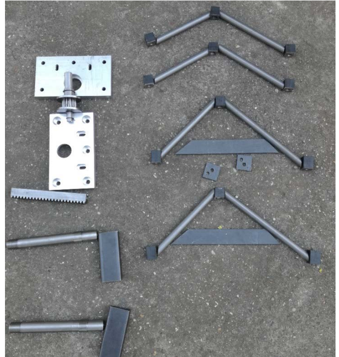
Fig. 20. Prefabricated elements of the front axle and steering gear before welding, drilling and assembly
